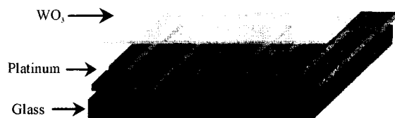
Fig. 1 Structure of the Sensor element
